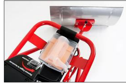
Battery withdrawal without tools
